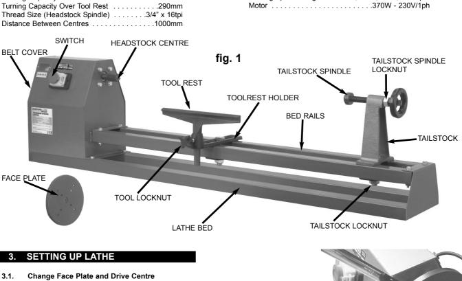
3.1.1. Unscrew the face plate (anticlockwise) while holding the headstock spindle using the spanner provided (Fig. 2).
