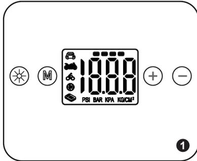
6.5.1. Press the LED light button
