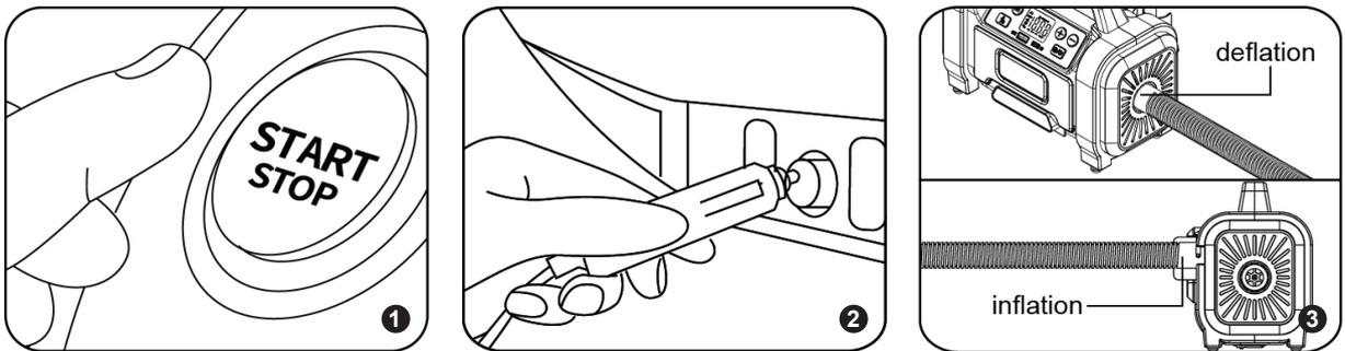
Step 1. Start the car engine before plugging in the power cord.
