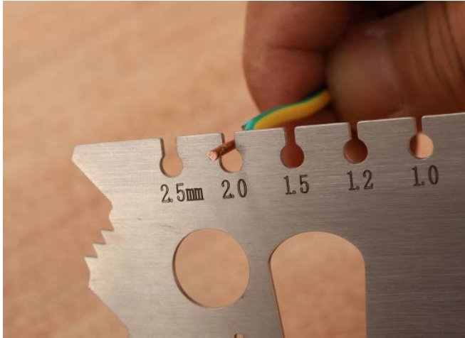
Wire Diameter Measuring
