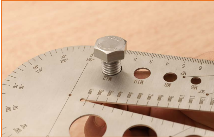
Gage Holes Measure the Bolt Thread
