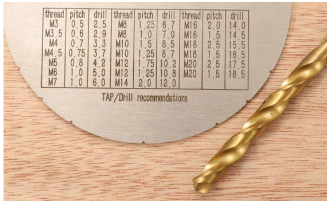
Select Right Size Drills for Different Thread Holes
