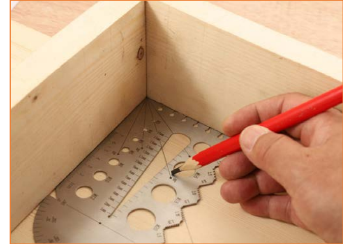
Marking Line Measure Angle 15°, 30°, 45° and 60°
