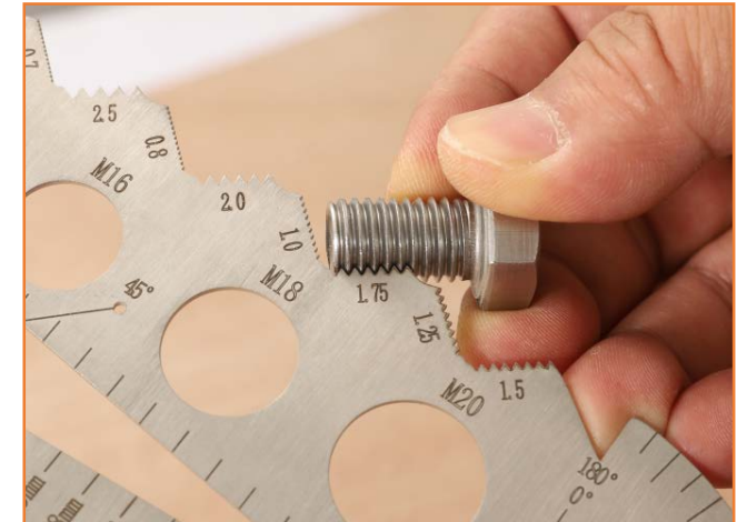
Pitch size Measure the thread
