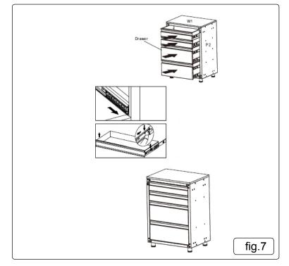
N.B. Maximum weight limit drawers:- 25Kg Maximum weight limit cabinet:- 150Kg
