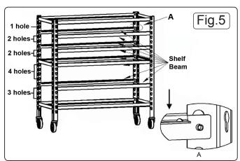
4.8 Starting at the bottom place the wire shelves into the frame ensuring the shelves for the larger bins are at the bottom and the shelves for the smaller bins are at the top. Place the flat wire
