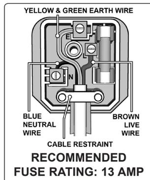
Double insulated products, which are always marked with this symbol
