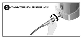
**4.1 Connecting the high pressure hose.** Remove and discard the transit plug from the water 'out' connector on the lower front of the machine (see fig.1). Attach the high pressure hose as indicated in fig.2 ensuring that the connector is tight.
