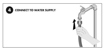
**4.2 Connecting the water supply.** Screw the hose connector to the water inlet on the machine (see fig.3). Use a reinforced hose pipe with an internal diameter of 1/2" and connect to the mains water supply as indicated in fig.4.
